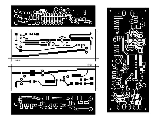
Except for the demodulator board all remaining modules require shielding. The frequency synthesizer is installed in one brass frame while the RF front end and IF amplifier are installed in another brass frame. The geometry of all brass frames is selected to keep any internal resonances high enough to avoid any need for microwave absorbers:
