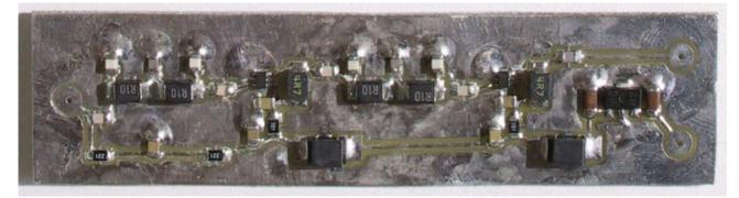
The third INA-52063 amplifier is connected to a FM demodulator built around an IAM-81008 analog multiplier. The output of the FM demodulator is limited and converted to TTL levels using 74HC02 logical gates. The demodulator module also includes the modulator driver 74HC125 and the RX/TX supply switch logic:
