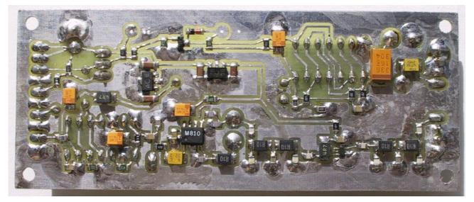
Both microwave boards are microstrip circuits (25mmX80mm and 20mmX80mm) built on 0.5mm (19mils) thick Ultralam 2000 teflon laminate. The remaining boards (twice 20mmX80mm and 40mmX100mm) are single-sided FR4:
