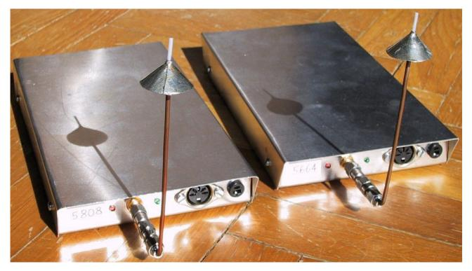
The microwave part of the synthesizer includes a VCO operating around 2.9GHz and a frequency doubler to 5.8GHz:
