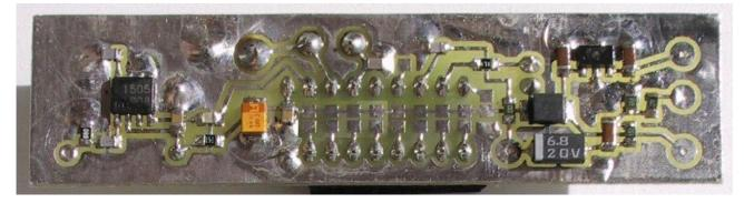
The RF front end includes a single HEMT MGF4918D. During transmission the HEMT operates as an amplifier with conventional DC drain bias. During reception the drain is not biased so that the HEMT operates as a passive mixer. An INA-03184 MMIC is used as the IF preamplifier. A bias network is provided to supply additional amplifiers through the antenna connector:
