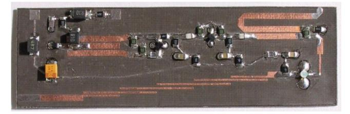
The digital part of the synthesizer includes a  $\mu PB1505$  prescaler and a MC145106 PLL chip supporting frequency steps of 24MHz selected by solder jumpers on the PCB:
