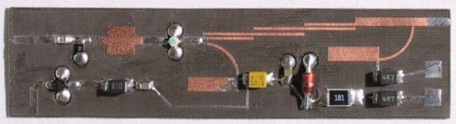
The INA-03184 is followed by three INA-52063 amplifiers in the IF chain. Two INA-52063 amplifiers are located in the IF amplifier module:
