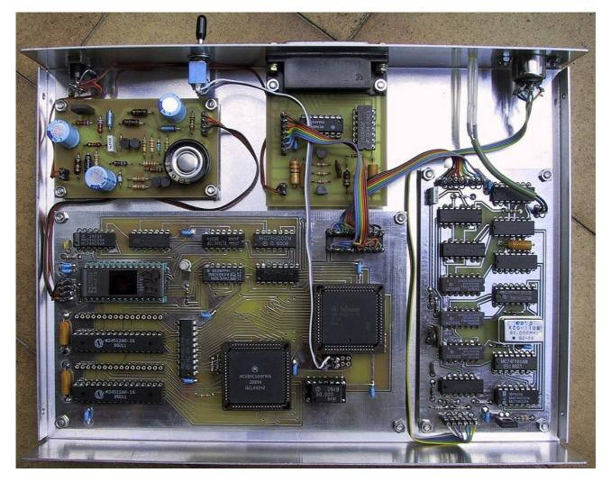
The power supply and the RS-232 interface are the same as in my old 1.2Mbps TNC design. The 10Mbps scrambler is designed with conventional 74HC... logic:
