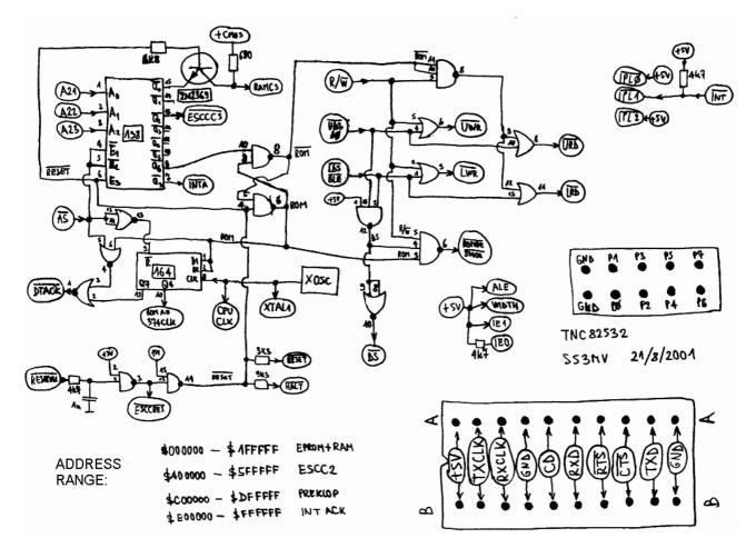
The data-bus width is 16 bits except for the EPROM and the latter is only used at power-up. The components of the 10Mbps TNC are installed on a 100mmX160mm double-sided PCB:
