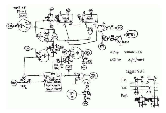
The clock recovery requires a fast DPLL. The latter works at a clock frequency of 80MHz and is designed with a single fast component (74F161 counter), while all other logic is from the 74HC... family:
