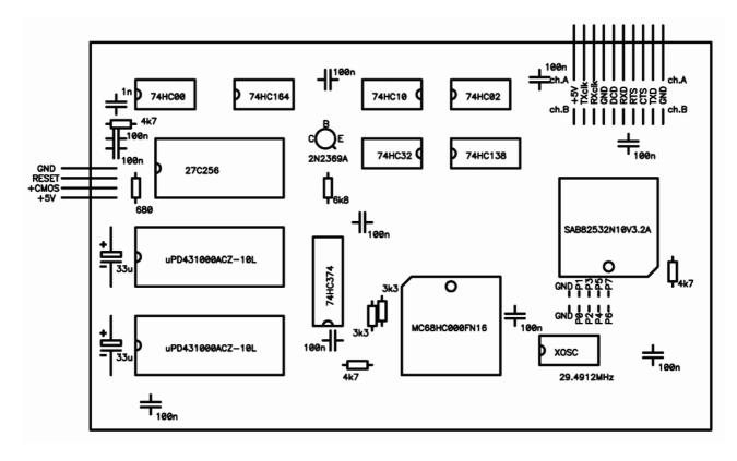
The two serial channels of the SAB82532N10V3.2 can be used in different ways. In the described TNC, the channel "A" is used for high-speed HDLC to the 10Mbps radio, while the channel "B" is used for conventional RS-232 asynchronous communication up to 921.6kbps. The parallel port is used to select the RS-232 speed and for circuit checkout. <br>
