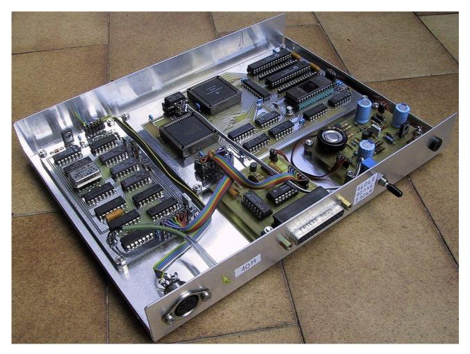
The SAB82532N10V3.2 allows a system clock up to 33MHz. The MC68HC000 in the PLCC-68 package can usually be overclocked reliably up to at least 40MHz. A full-duplex operation with short packets that fit in the SAB82532's FIFOs is possible up to 33Mbps. Reliable full-duplex operation with longer data frames is possible up to 12Mbps.
