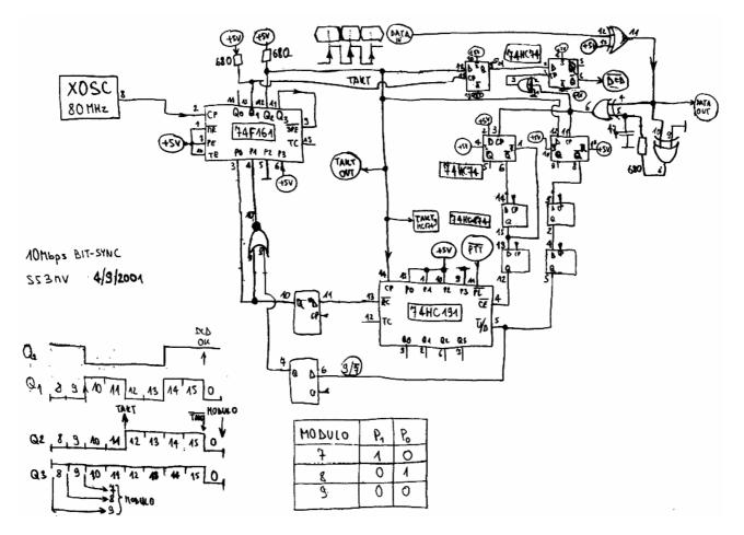
The 10Mbps scrambler/clock-recovery circuit is built on a 60mmX120mm double-sided PCB (values in brackets for 1.2288Mbps operation):
