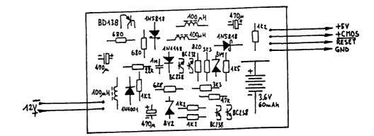
Fig. 11 - Power-supply component location.
