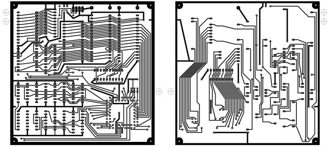
Fig. 3 - TNC double-sided printed-circuit board.
