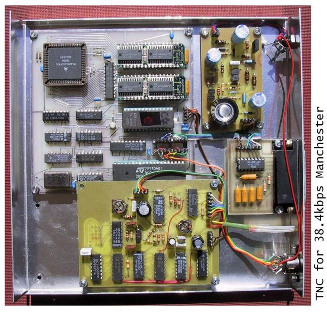
For the network developer or sysop, the megabit TNC may have advantages too. Most important, one single user can never get all of the capacity of a megabit channel thanks to his/her RS232 bottleneck, thus blocking the access to other users. A megabit TNC also allows testing new protocols in the network without changing the actual user terminal software running on host computers.
