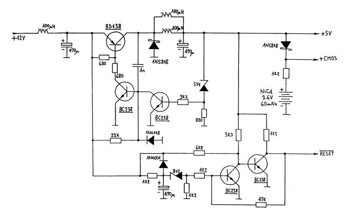
Fig. 9 - Power supply and reset circuit.
