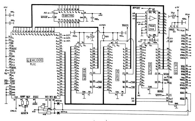
Fig. 1 - CPU, memory and serial port.
