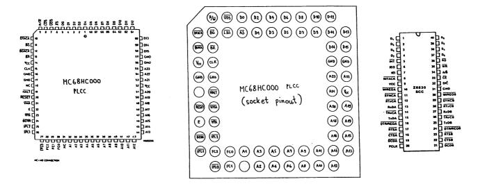
Fig. 5 - CPU and serial-port pinouts.
