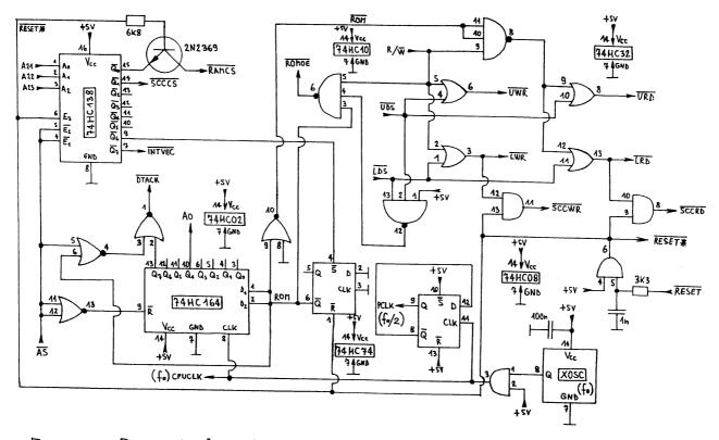
Fig. 2 - Bus interface logic.
