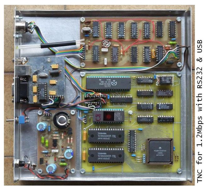
Finally, the described megabit TNC equipped with CMOS parts can also work as a simple, very low-power digipeater already with the currently-available KISS software. The overall current consumption of the TNC is about 100mA at 12V. Adding about 200mA for the 23cm PSK transceiver, the whole digipeater can be powered with a 50W solar panel and a large "diesel" car battery.
